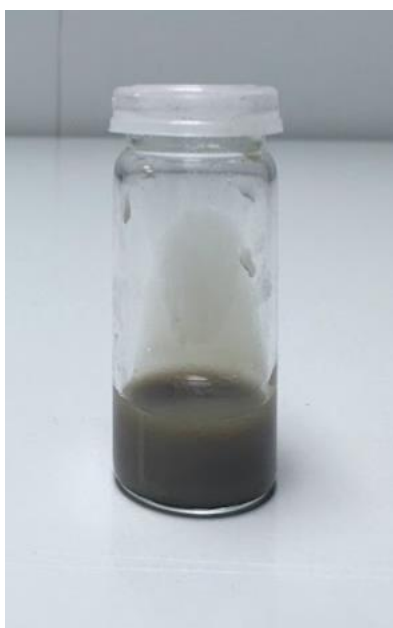
Figure 3.26: PVA: InSe-H 2 O, prepared after 1h at 75°C, under stirring at 650 rpm.
