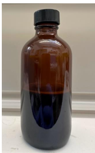
Figure 3.25: InSe-solvent solution sonicated in DI H 2 O for 15 h.
