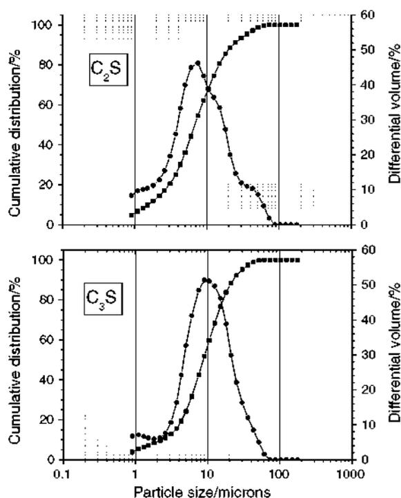
Fig. 1 Particle size distribution for anhydrous C<sub>3</sub>S and C<sub>2</sub>S
