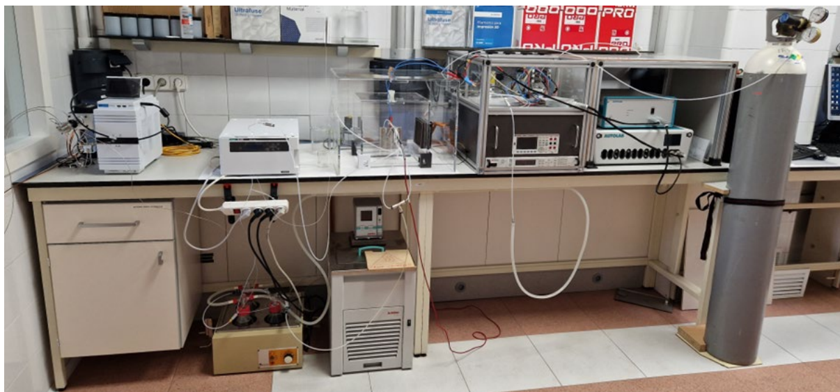
Figure 3.20: Photograph of the Methanol Electrolysis Cell (MEC) and Direct Methanol Fuel Cell (DMFC) test bench designed and built in this thesis and used for MEC tests
