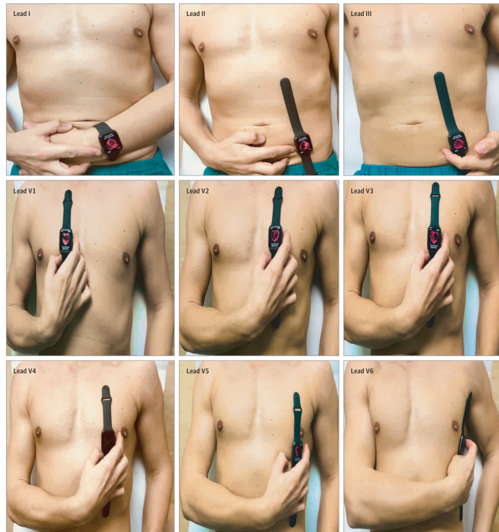
Figure 1.4: The positions of the smartwatch to obtain 9-lead ECGs. Source: [6].
