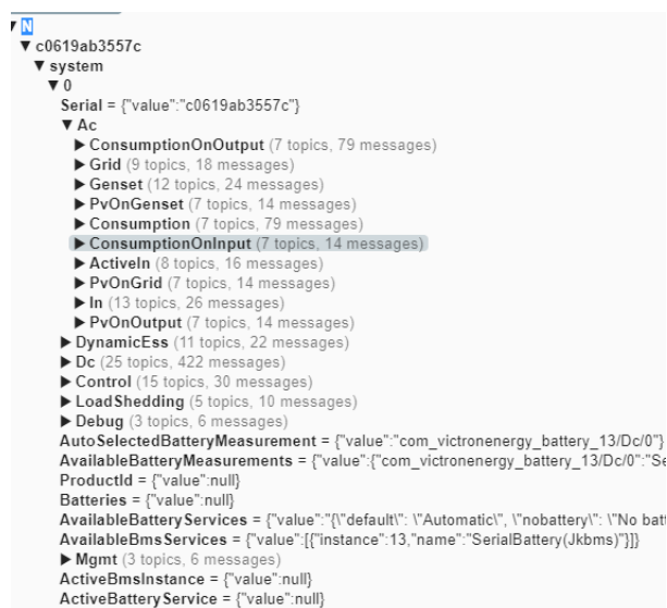
Figure 5.5: MQTT messages (only few of) that are being transacted on the system every second.
