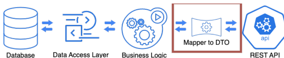
Figure 4.13: Data encapsulation strategy with mapper as a reference to the endpoints by [Buddy(2024)].
