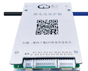
Figure 5.1: JK BMS with unwired socket connections by [Nkon(2022)].
