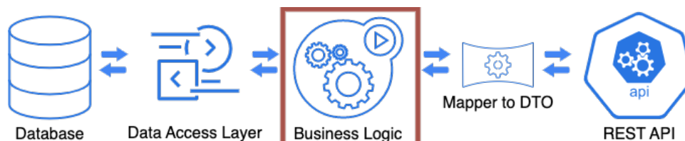
Figure 4.11: Data encapsulation strategy with business logic as a reference to the endpoints by [Buddy(2024)].
