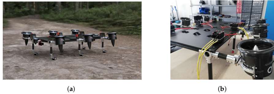
Figure 2. A brief schematic of Fan Hopper’s designed model; (a) the configuration with components installed as a whole; (b) the incident angle of the ducted fan.
