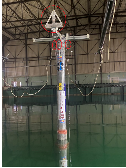
Figure 5.6: The spar model in testing position with the instrumentation circled in red.
