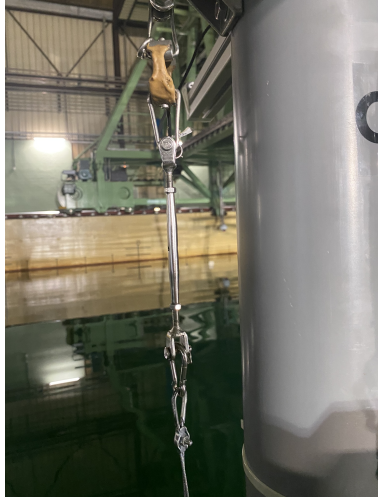
(a) Detailed view of one of the load cells with the turnbuckle.
