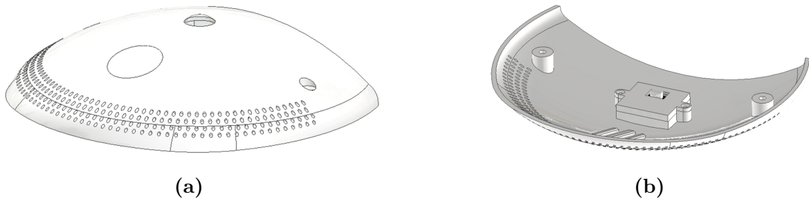
Figure 4.18. Details of the head top panel: (a) Top view, (b) Bottom view.
