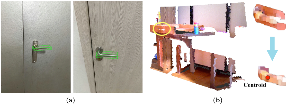
Figure 2.11. Handle detection and localization: (a) Handle detection through CNNs [82], (b) RANSAC algorithm application [81].
