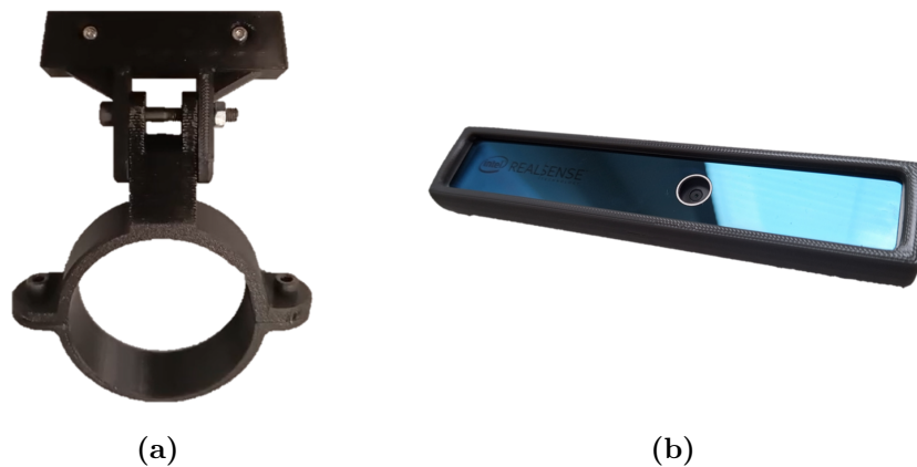
Figure 4.25. 3D-printed camera components: (a) Support, (b) Cover.
