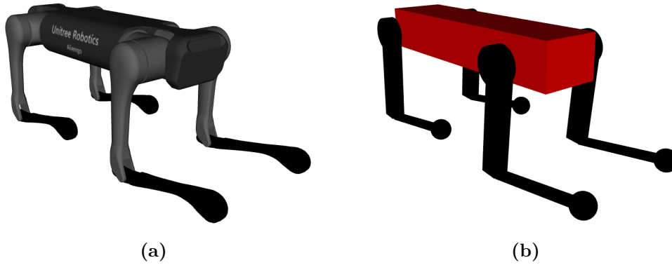
Figure 4.2. AlienGo quadruped URDF model: (a) Geometric model, (b) Collisions model.
