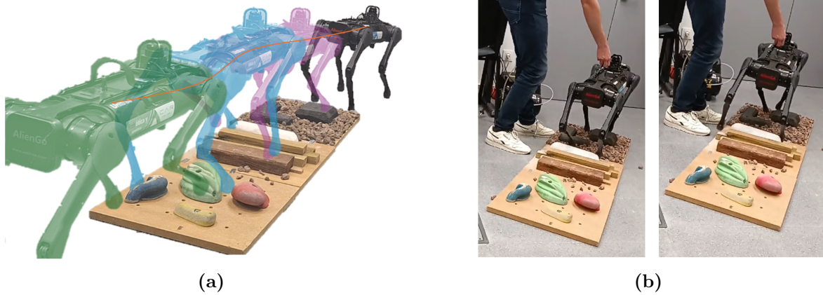
Figure 5.21. AlienGo hardware testing: (a) Followed path, (b) Safety textile handle.
