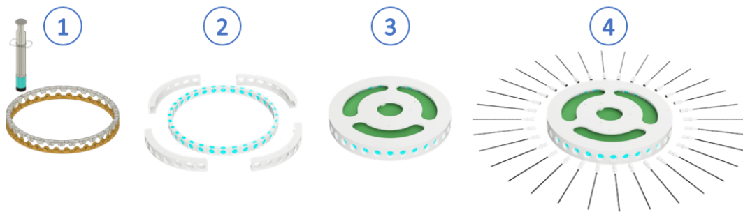
Figure 3. Whisker disk assembly procedure. First, the silicone base is prepared by injecting the mixture into the plastic rings. Next, the silicone rings are clamped and assembled into the disk structure with a set of screws. Finally, the PCB is installed, and the whiskers are inserted through the silicone ring until the spherical contact reaches its position.
