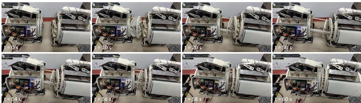
Figure B.3: Self-assembly coupling maneuver between two mobile modules.
