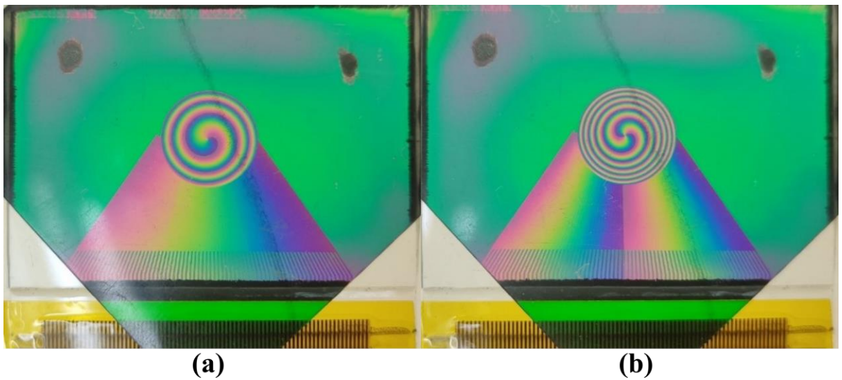
Figure 6.16: Manufactured SDL with half inch active area diameter configured with different topological charges: a) l = 1 . b) l = 2 .
