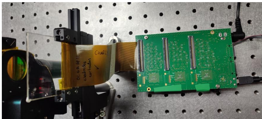
Figure 3.5: ADTelecom electronic driver.
