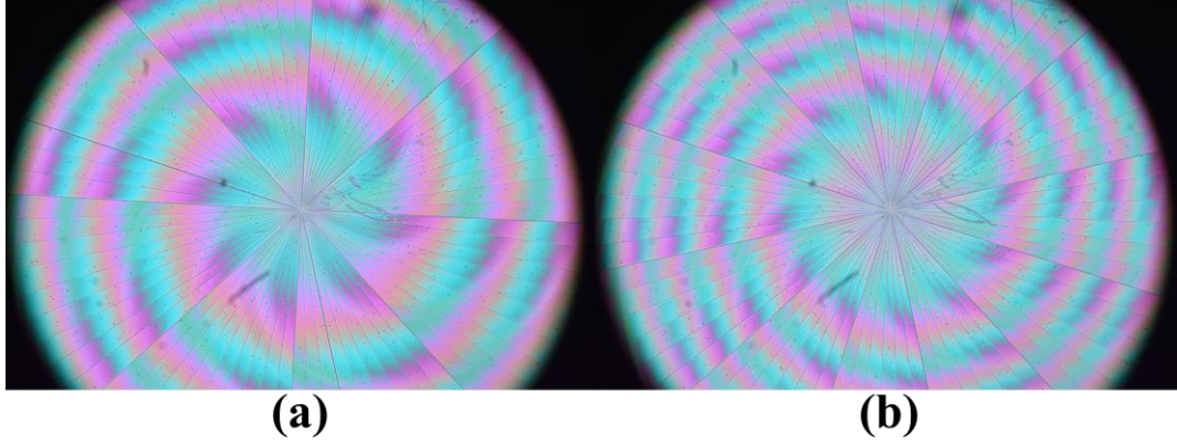
Figure 6.18: Micrographs under white illuminations showing under crossed polarizers the SPP and SDL assembly for different configurations. a) l_{SDL} = 8 , l_{SPP} = -8 . b) l_{SDL} = 10 , l_{SPP} = -10 .
