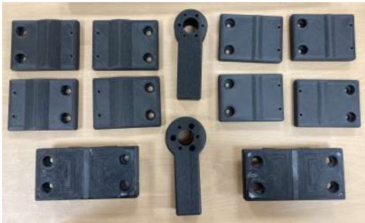
Figure 4.18: Parts made of ABS-CF10
