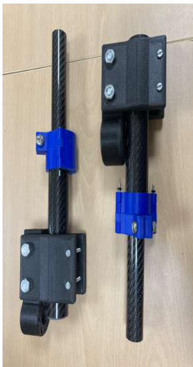
Figure 4.20: Subassemblies for the arm and forearm of the exoskeleton
