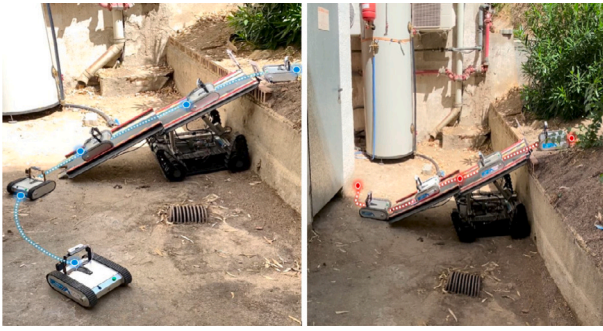
Fig. 6. Ascending and descending for environment exploration using collaborative robots in environment defined by Fig. 3.
