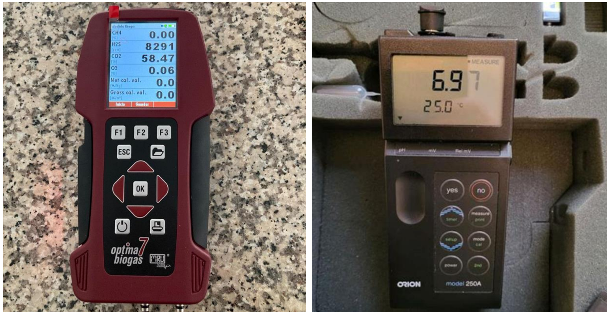
Figure 36: The MRU Optima 7 biogas characterisation meter (left) and Orion 250A pH measuring device (right).
