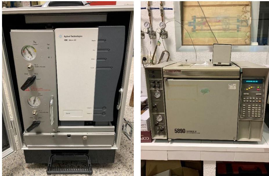
Figure 13: Gas chromatographs used for permanent gas characterisation (left) and sulphur content analysis (right)
