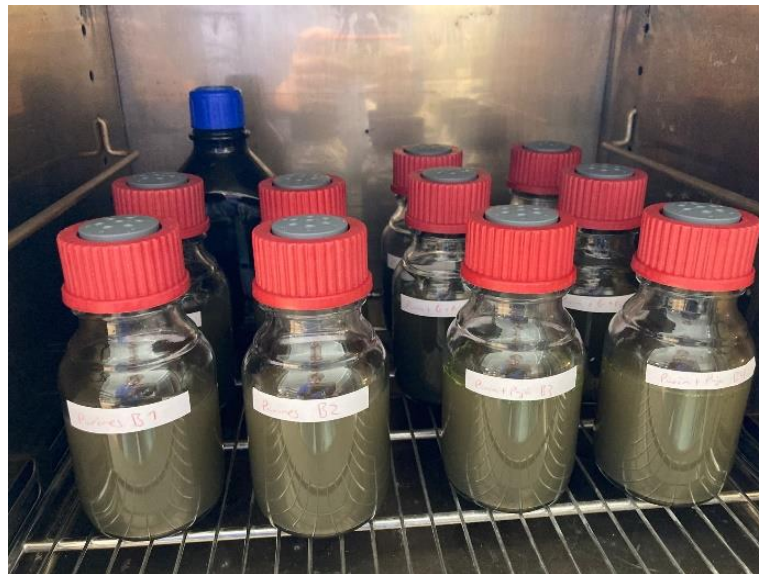
Figure 11: Batch reactors used. Image taken from the oven at 37 °C, simulating mesophilic conditions.
