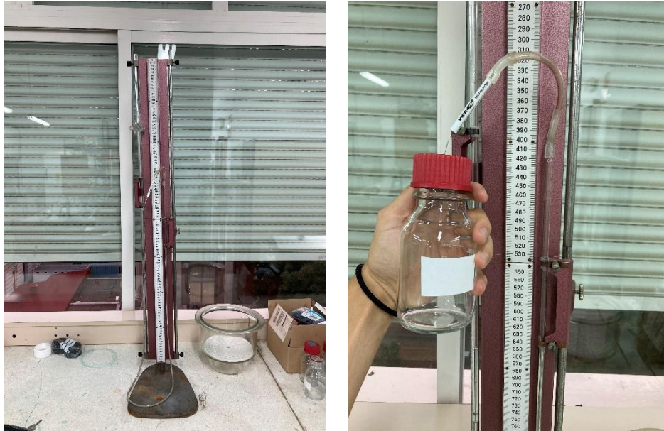
Figure 12: U-tube pressure measurements (left) and needle system used to pierce the rubber septum (right)
