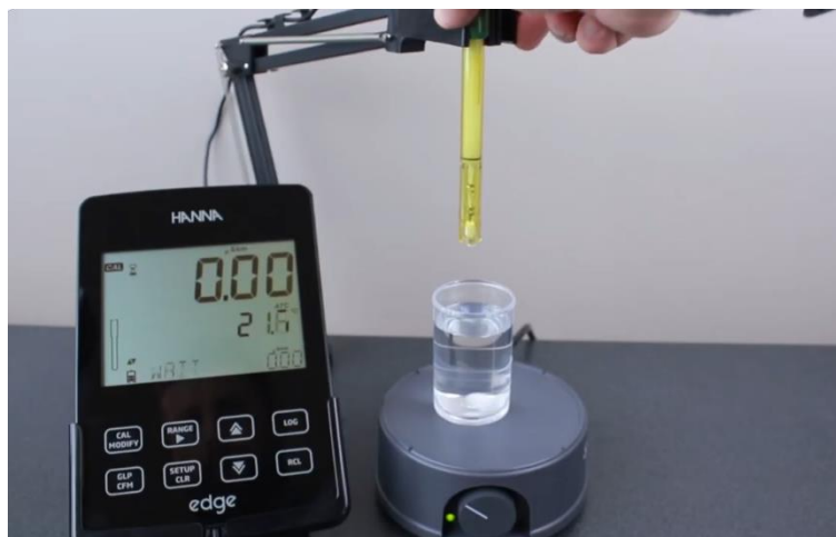
Figure 28: A sample pH-meter used for pH sampling of digestate (Image credits: Hannah Instruments)
