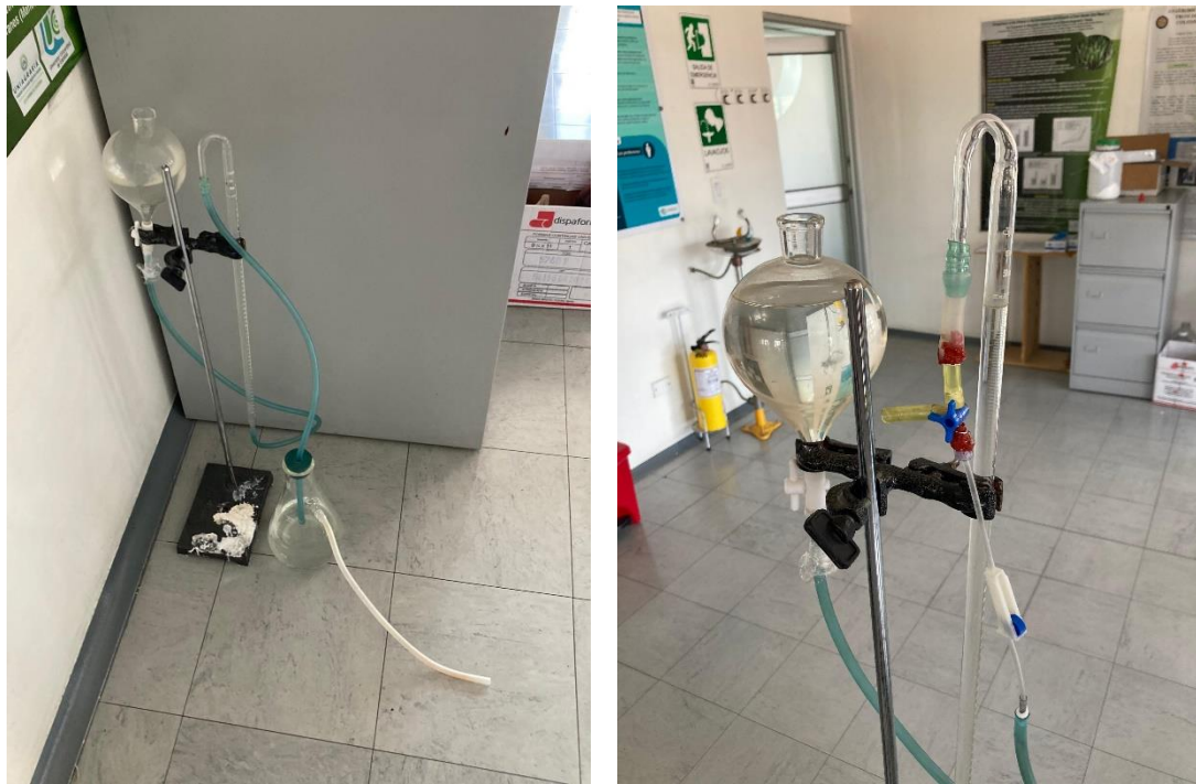
Figure 26: Water displacement apparatus (left) and three-way valve (right)
