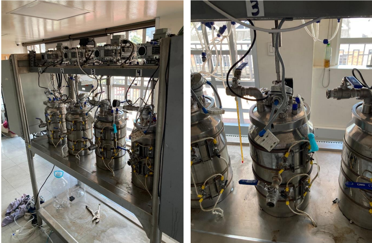
Figure 24: The reactor installation at the Universidad Cooperativa de Colombia, which hold a specialist laboratory dedicated to the research and development of AD and fermentation technologies. Left: whole reactor assembly. Right: detail view of one reactor. Experimentation in Chapter 6 was conducted with these reactors.
