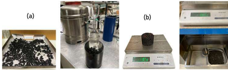
Figure 3.18: Volumetric characterization of the test to evaluate a) Apparent density (Gmb), and b) maximum density (Gmm). Source: Author's elaboration.
