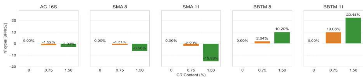
Figure 4.25: Effect of CR on the threshold of BPN=52.
