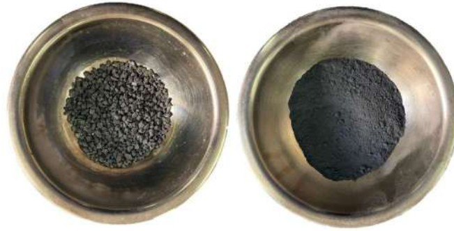
Figure 3.7: Electric arc furnace slag (EAFS).
