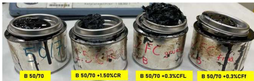
Figure 3.57: Binder's base, and binders with crumb rubber, large carbon fiber, and fine carbon fiber. Source: Author's elaboration.
