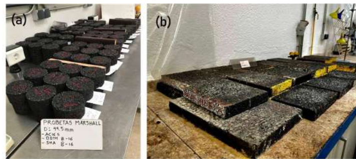
Figure 3.15: a) Cylindrical and b) slab specimens manufactured. Source: Author's elaboration.
