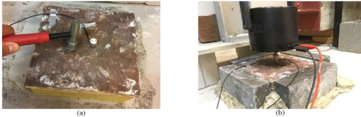
Figure 2.65: a) Hammer method and b) Shaker excitation was used to evaluate the dynamic stiffness.(Urbán & Roozen, 2020).
