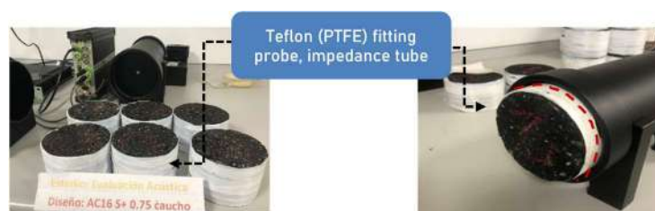
Figure 3.60: Pre-conditioning specimens with PTFE on their lateral surface. Source: Author's elaboration.
