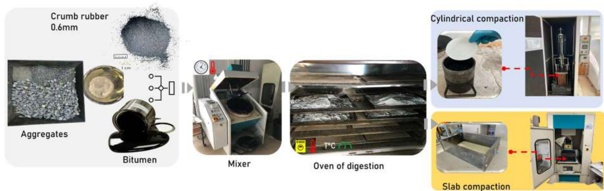
Figure 3.14: Process to digestion and compaction of asphalt mixtures cylindrical, and slab samples. Source: Author's elaboration.
