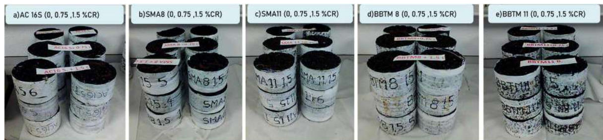
Figure 3.62: Rubberized bituminous specimens with a lateral band of PTFE, a) AC 16 S, b) SMA 8, c) SMA 11, d) BBTM 8 B, and e) BBTM 11 B. Source: Author's elaboration.
