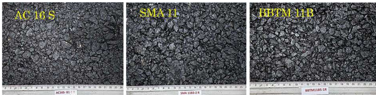
Figure 3.3: Different surface texture of the asphalt mixtures under study. Source: Author's elaboration.
