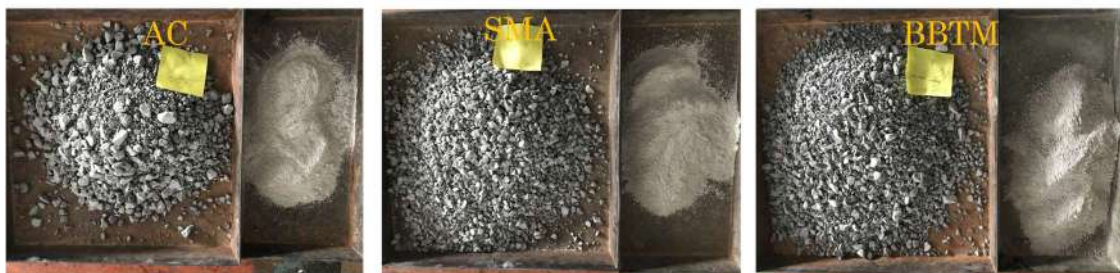
Figure 3.11: Gradation for different asphalt mixtures. Source: Author's elaboration.
