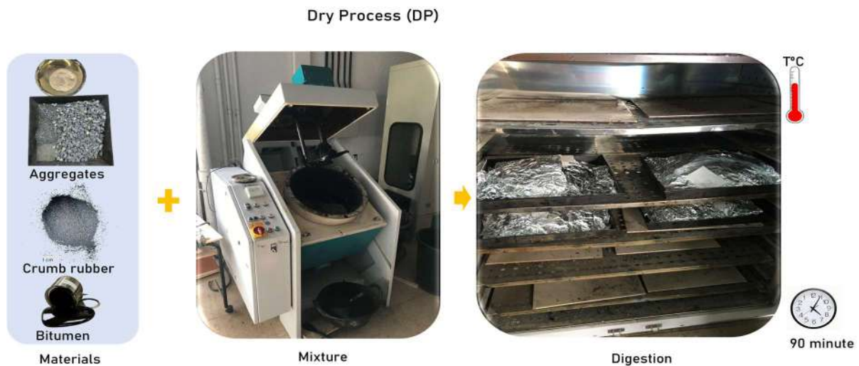
Figure 3.13: Digestion by Dry process. Source: Author's elaboration.
