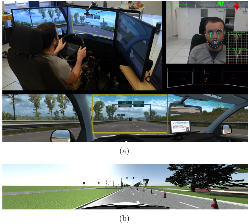
Figure 6.9: Integration of DMS pipelines in driving simulation: (a) Driver monitoring captures using driving simulator, (b) PreScan virtual world at AHiDA-M use case simulation.
