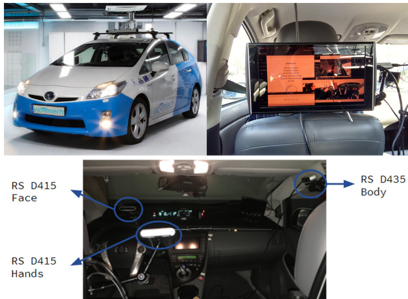
Figure 6.10: Vehicle equipped with interior cameras (Intel RealSense D400) for face, body, and hand monitoring, alongside perception and localization devices (Velodyne HDL-32, 4 Sekonix 100° cameras, xNAV550, uBlox), and broadcasting mechanisms to display demo images outside the vehicle.
