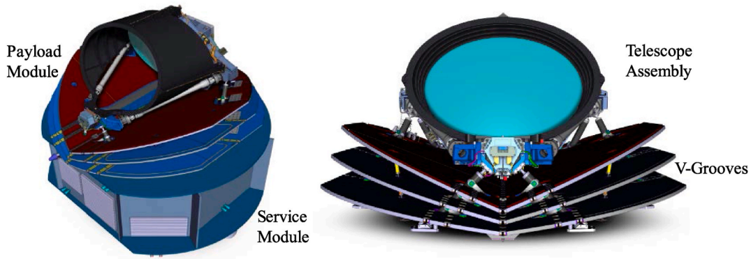
Fig. 1. ARIEL spacecraft overview (left) and PLM overview (right).
