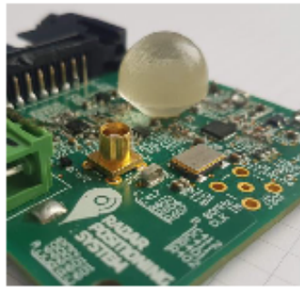
Fig. 5 Plastic lens attached to the radar SoC
