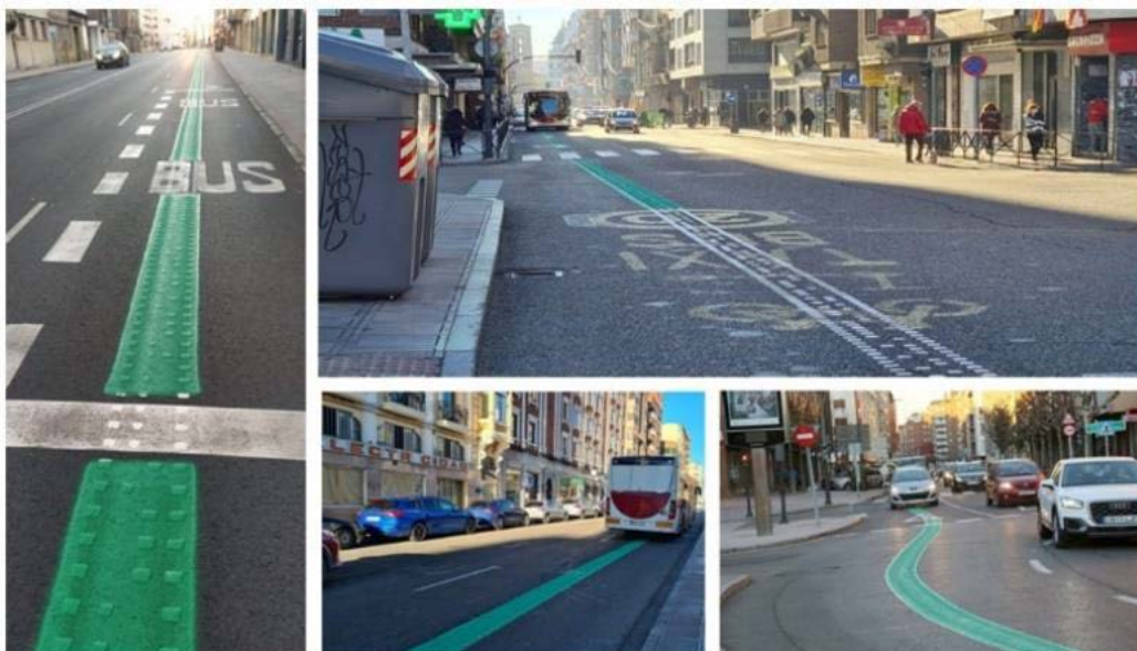
Figure 21 Coded track deployed in Leon city to support public transport
