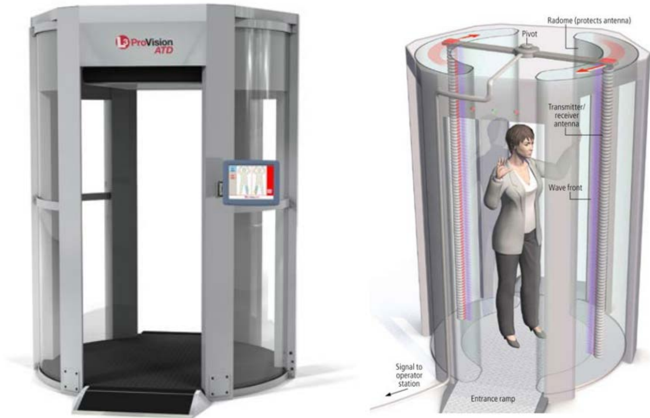
Figure 4 Millimeter-wave portal for concealed object detection
