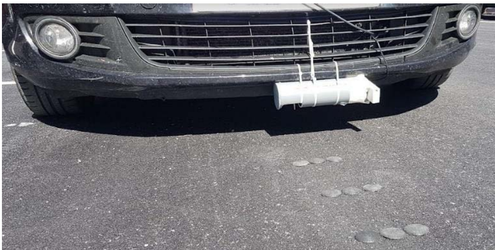
Figure 32. Onboard radar setup
