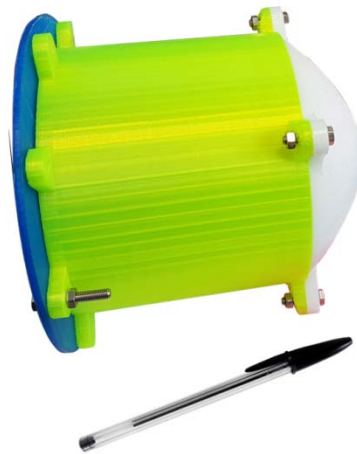
Figure 9. 120 GHz lens prototype
