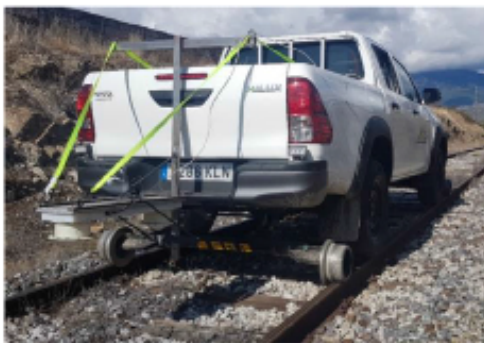
FIGURE 13 (Left) Assembling of the equipment for developing test 1 on railway track 1.
