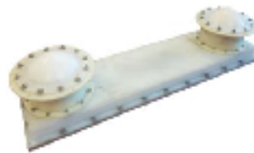
Fig. 3: Two radar sensors for scanning the ground shape
