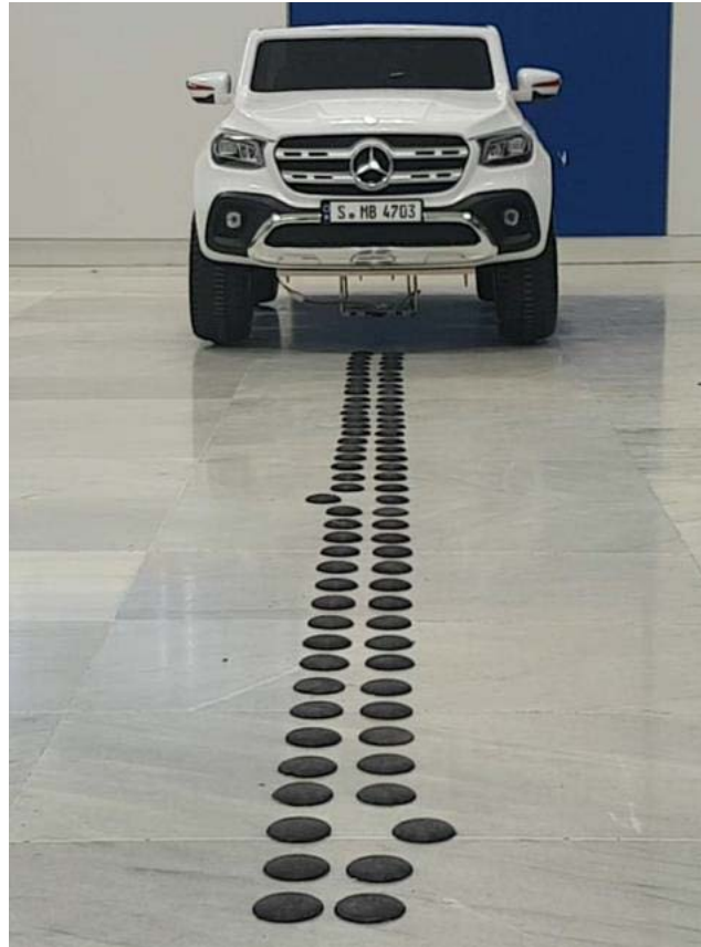
Figure 26. Low speed vehicle guidance track setup
