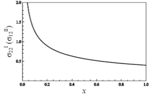
Figure 5: Variation of normalized phonon tensile (shear) stress along the interface ahead of the crack tip under remote Mode I (Mode II) loading conditions.
