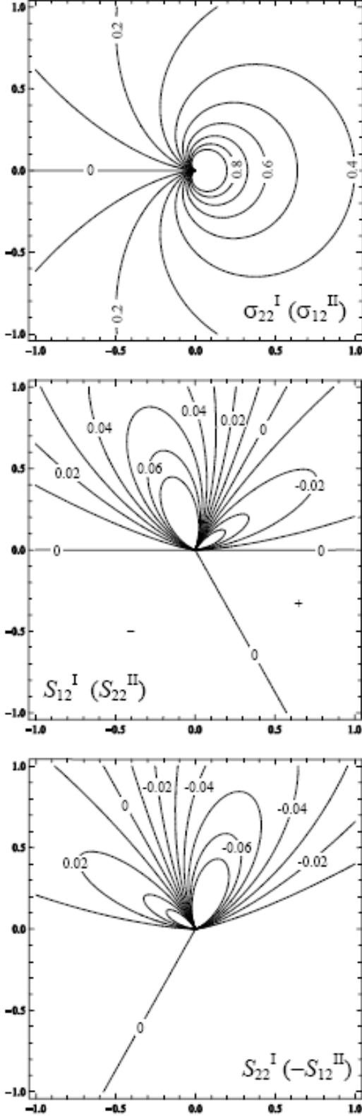
Figure 4: Contours of normalized phonon and phason stress fields for a semi-infinite rectilinear crack under remote Mode I (Mode II) loading conditions, for  $\lambda^{(1)} = \lambda^{(2)} = 85GPa$ ,  $\mu^{(1)} = \mu^{(2)} = 65GPa$ ,  $k_1^{(1)} = k_1^{(2)} = 0.044GPa$ ,  $k_2^{(1)} = k_2^{(2)} = 0.0396GPa$ ,  $\chi^{(1)} = 5$  and  $\chi^{(2)} = 0.1$ .
