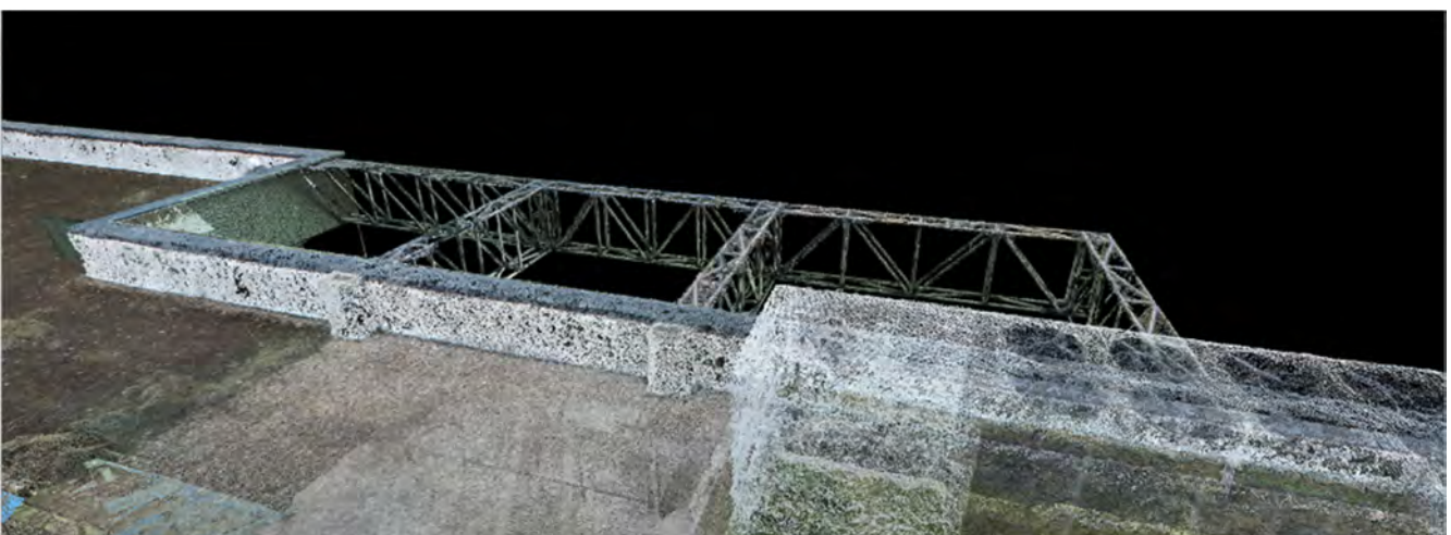
Figure 12. Metal elements from the merged dataset—Leica Cyclone—view based on the RGB code taken from the images.
