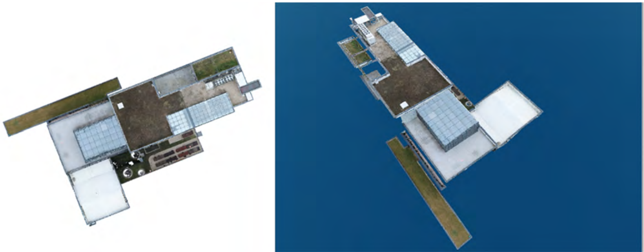
Figure 9. The results obtained after filtering the dense point cloud based on altitudes (terraces and ceilings).
