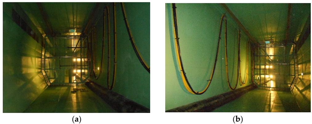
Figure 3. Interior of the cargo tanks and transverse bulkhead arrangement to facilitate unloading operations. (a) port tank, (b) starboard tank.
