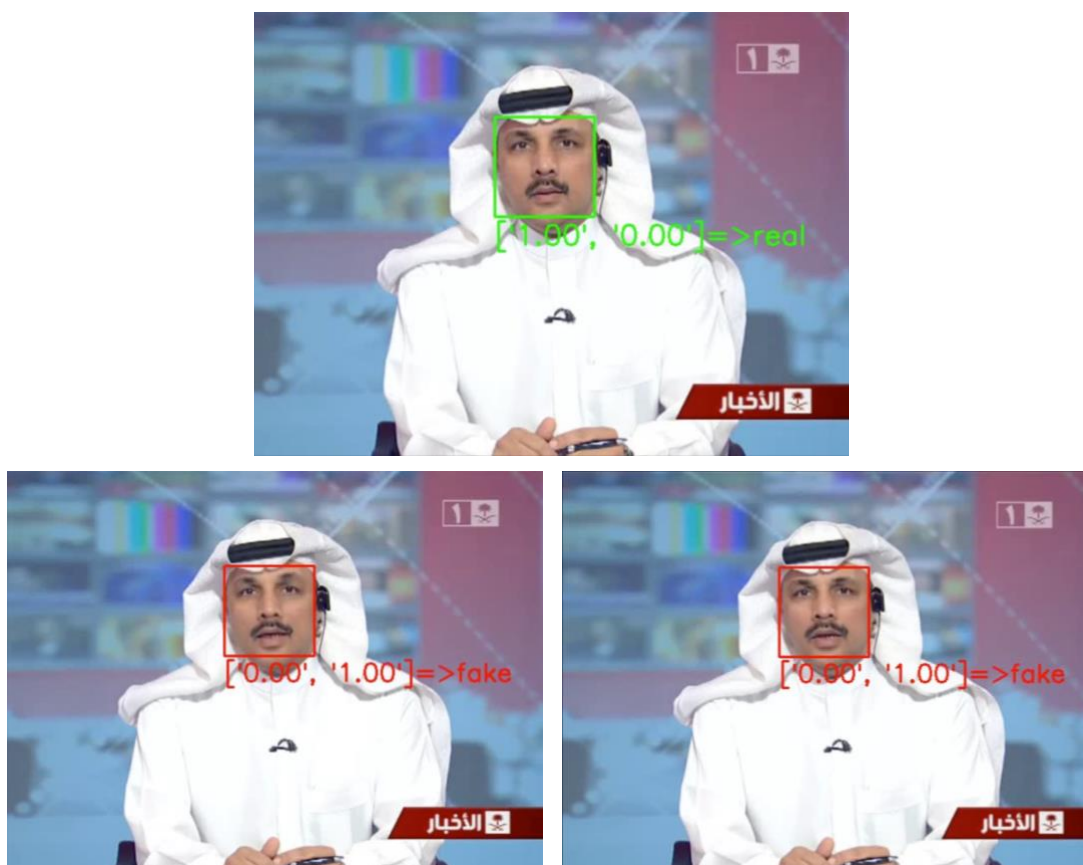
Figure 5: First frame of the first video from the original (upper), Face2Face (left) and NeuralTextures (right) videos, all with raw quality. The bounding boxes and predictions can be appreciated
