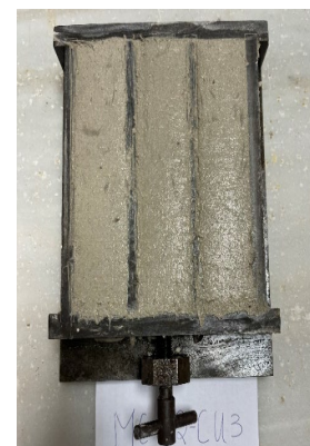
Fig. 5. Filling and screeding the metal moulds. Source: Photographs by author.
