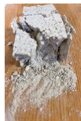
Fig. 7. 180-day compressive test. Source: Photograph by author
