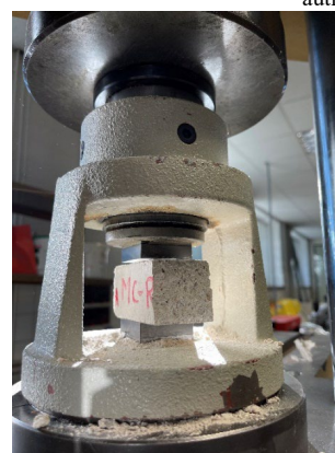
Fig. 7. 180-day compressive test. Source: Photograph by author
