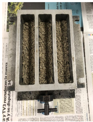
Fig. 5. Filling and screeding the metal moulds. Source: Photographs by author.
