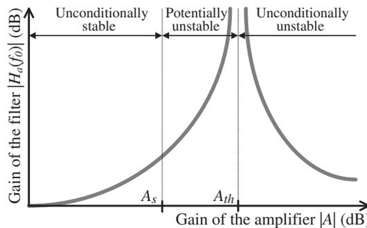
**Figure 6.** Transfer function (4) of a first-order active filter as a function of the gain of the amplifier and typical stability regions.
