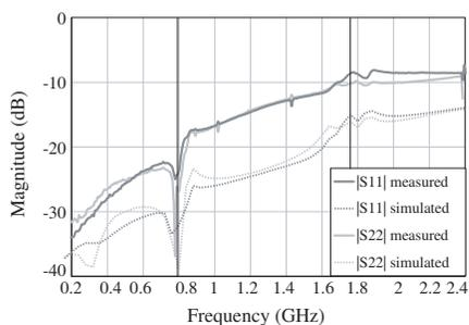
**Figure 19.** Reflection coefficients of the third-order active filter.
