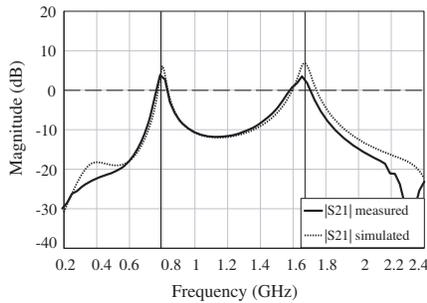
**Figure 11.** Transmission coefficient of the first-order active filter.
