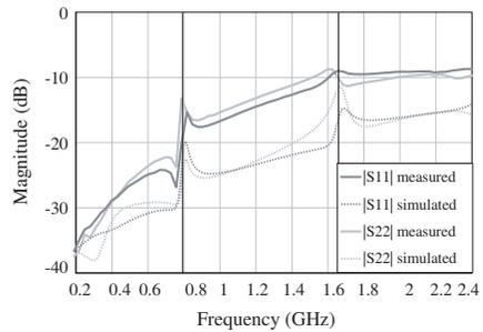
**Figure 12.** Reflection coefficients of the first-order active filter.
