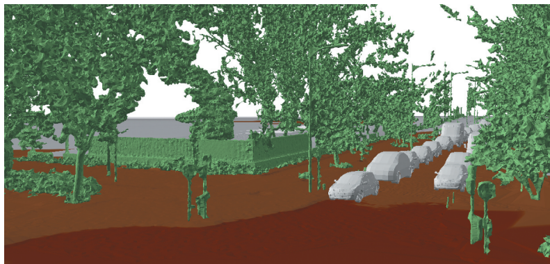
Figure 10. 3D model of the intersection with Novais Street busy. Automobiles are modeled as gray elements, aboveground elements in green and the DTM in shades of brown.
