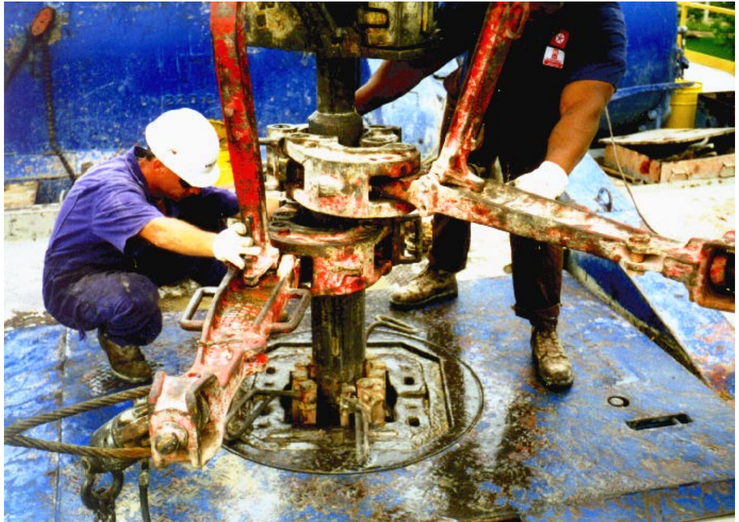
Position of the hand wrenches to tighten the threaded joint
