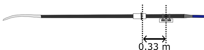
Fig. 13: Representation of the prototype reference distance on the oar's tube.
