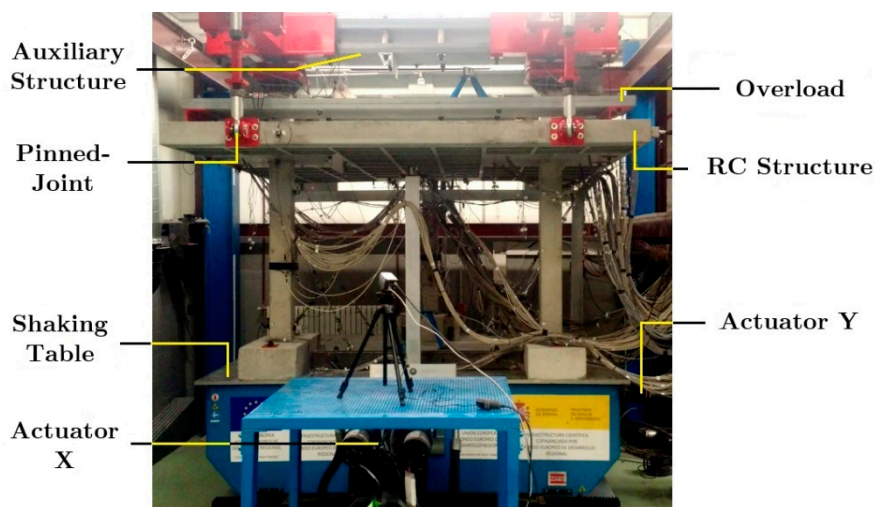
Figure 3. General setup of the seismic test: Shaking table of the Laboratory of Structures of the University of Granada (actuators X and Y), reinforced concrete (RC) main structure with overload, and auxiliary metallic structure.
