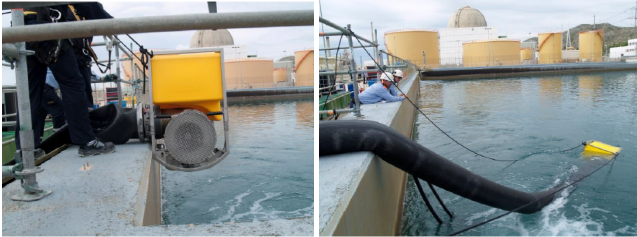
Figure 3.6: Submersible portable pump FLEX-SUP for use in FLEX strategies [ANAV, 2013]
