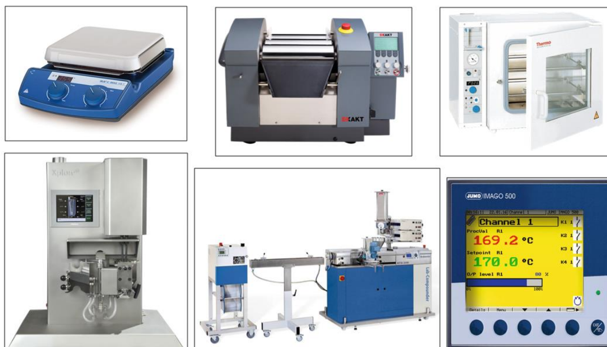
Fig. 3-1 lab devices. Above: from left to right are magnetic stirrer, three roll mill and vacuum oven; below: from left to right are micro compounder, twin-screw extruder and hydraulic hot press
