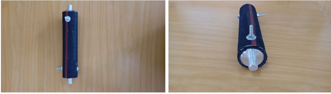
Figure 3.2: Piece of hose used in the tension test.
