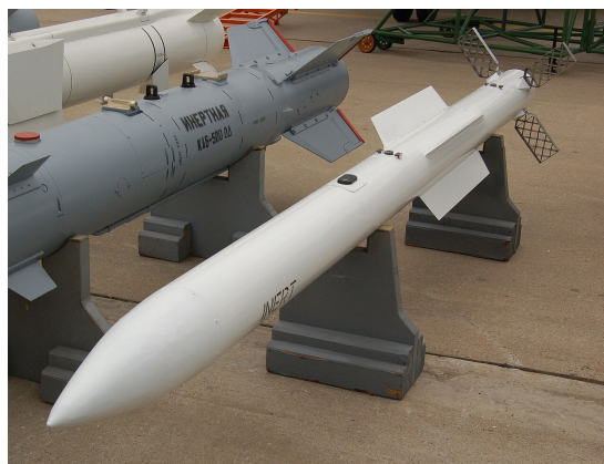
Figure 1.11: Folding grid fins of the R-77, extracted from santosh aerospace.blogspot.com .
