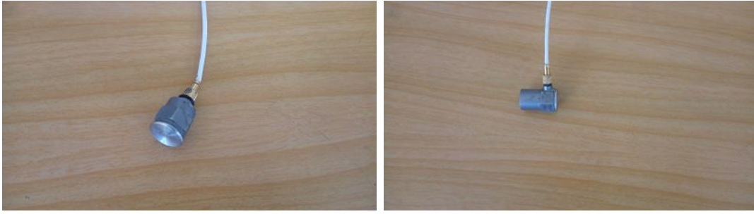
Figure 3.9: Accelerometers used in the vibration test. On the left side, Brüel & Kjær, and on the right side, PCB.
