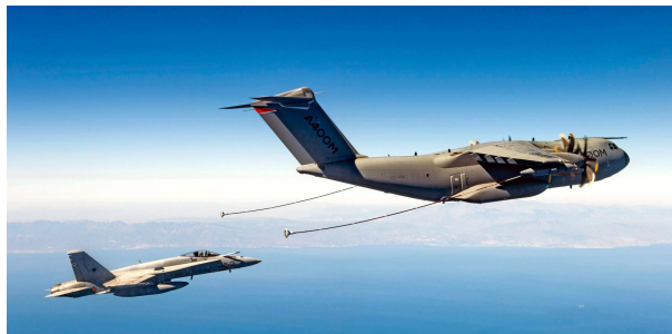
Figure 1.8: Aerial refueling process with hose and drogue system. Extracted from Naval Aviation News .
