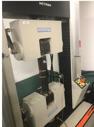
Figure 3.3: Piece of hose and tension machine before the test.
