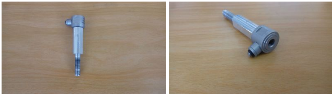
Figure 3.11: Load cell used in the vibration test.
