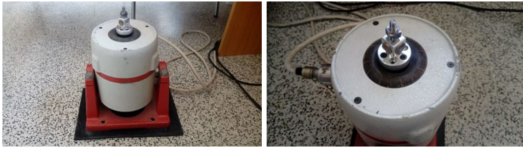
Figure 3.10: Shaker used in the vibration test.
