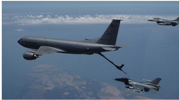
Figure 1.7: Aerial refueling process with flying boom system. Extracted from [Sahin, 2010].
