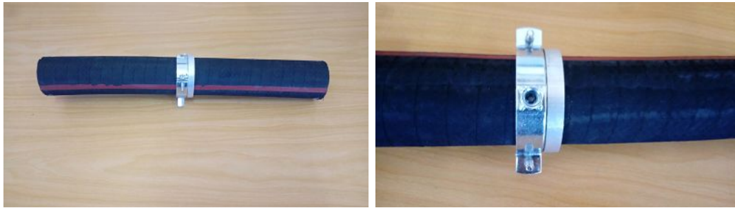
Figure 3.8: Piece of hose and clamping structures for the vibration test.
