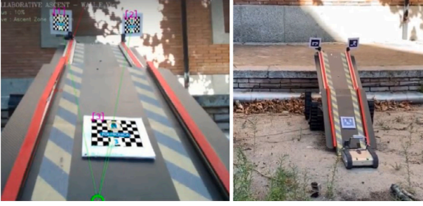
Fig. 4. Beacon detection system and estimation of distances-orientations.
