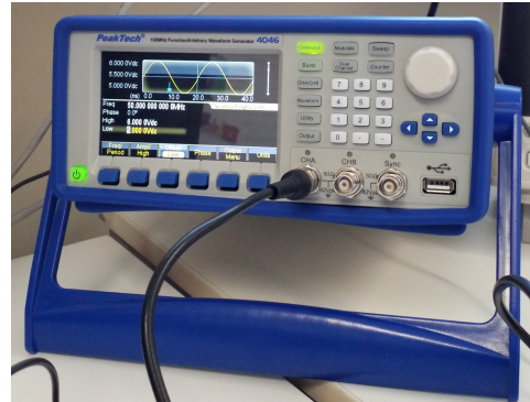
Fig. 4. Voltage modulation with PeakTech 4046 function generator
