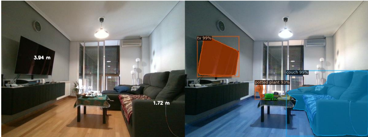
Figure 14 - Screen shot of the solution capturing the instances and their distances in the scene
