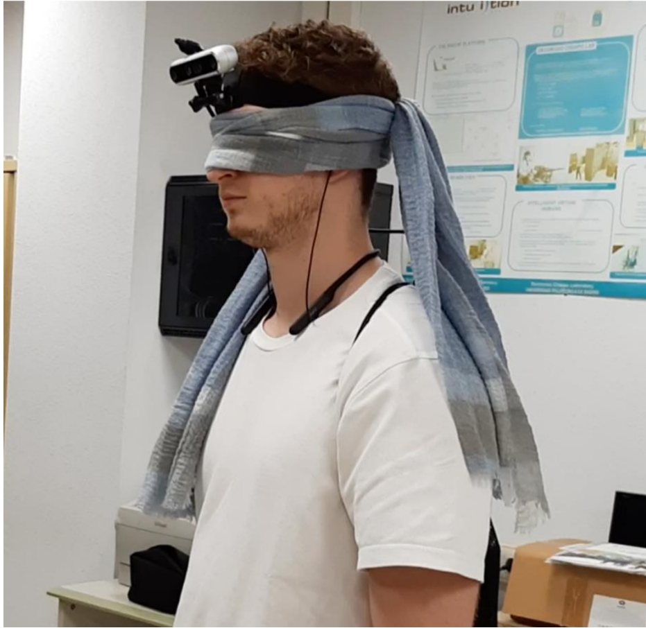
Figure 12 - A user wearing the solution including the backpack with the laptop, camera and the headphones
