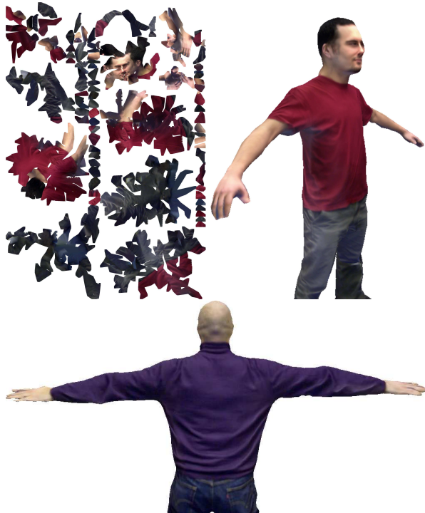
Figure 5: Top left: texture atlas resulting from the complete multi-texturing process. Top right: corresponding textured model. It is possible to see how discontinuities present in Figure 2 have been completely removed. Bottom: another reconstructed and textured model showing how folds in the pull-over are perfectly reproduced, even though the color information comes from different input images.
