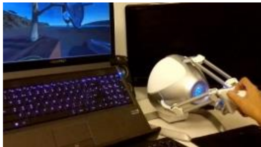
Figure 3: The haptic device used at ImmersArt to provide virtual touch to the user: the Novint Falcon.
