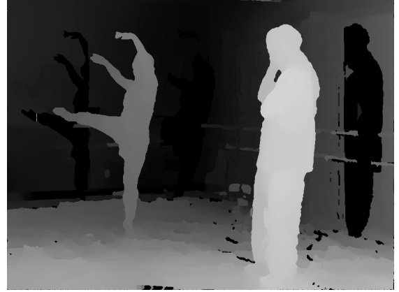
Fig. 5. Final depth map estimation on the virtual camera obtained from both reference cameras.
