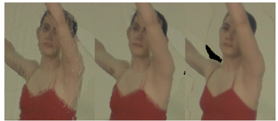
Fig. 9. Detail of foreground texture registration errors. Left to right: Wide baseline unfiltered forward mapping, wide baseline backward mapping, short baseline backward mapping.
