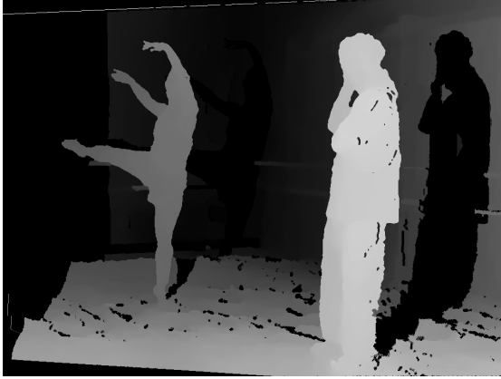
Fig. 4. Depth map estimation on the virtual camera obtained from only one reference camera after a filtering stage.
