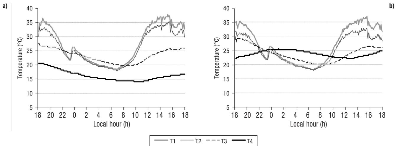
**Figure 6.** Stratification of temperatures around the plant: (a) RHF scenario (b) control scenario. T1: air temperature at a height of 1 m; T2: air temperature at a height of 0.5 m; T3: substrate temperature next to the roots; T4: soil temperature at the bottom of the plant pot (data collected on a single day in 2005).
