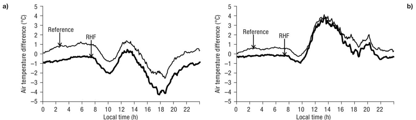
**Figure 4.** Air temperature difference between the inside air and outside air for an average day under both cooling scenarios (calculated from the data collected over 16 days during 2005). (a) Inside air temperature measured at a height of 0.5 m; (b) Inside air temperature measured at 1.5 m.
