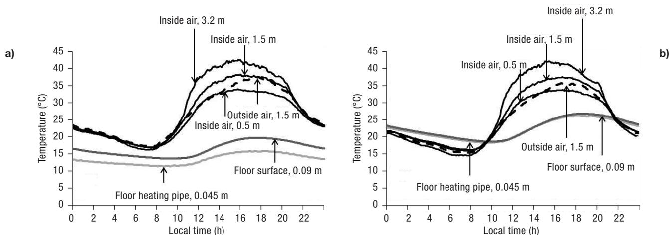
**Figure 3.** Stratification of greenhouse temperatures in (a) the RHF scenario (b) control scenario; results are for an «average day» (calculated from the data collected over 16 days during 2005).
