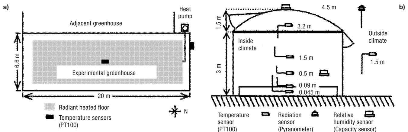
**Figure 1.** a) Plan view of the experimental greenhouse; location of the heated floor and the air-water heat pump. b) End view of the experimental greenhouse with the sensor system.
