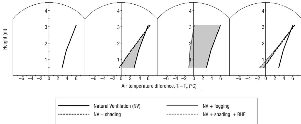
**Figure 5.** Experimental data: mean values for the critical period 13:00-17:00 h. Graph comparing the air temperature difference obtained from different cooling strategies,  $T_i - T_o$  (°C) at different heights. The shaded area shows the improvement of the cooling effect achieved with the addition of technologies.
