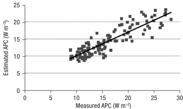
**Figure 9.** Validation of the heat pump model ( $r^2=0.78$ ,  $n=120$ ). Estimated APC vs. measured APC. Mean values for 5 days of the summer of 2006. Rated power consumption,  $34.1 \text{ W m}^{-2}$ .
