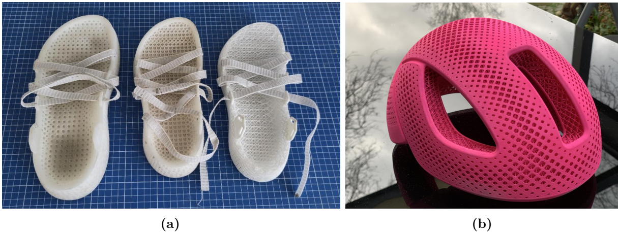
Figure 1.4: Shoesole and helmet prototypes made with lattice materials developed in the MOAMMM project.
