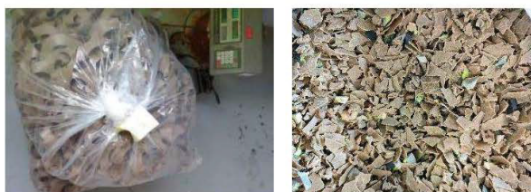
Figure 1: Remains of rubber sheet previously and once crushed to 5mm. Fuente: Elaboración propia (2022)
