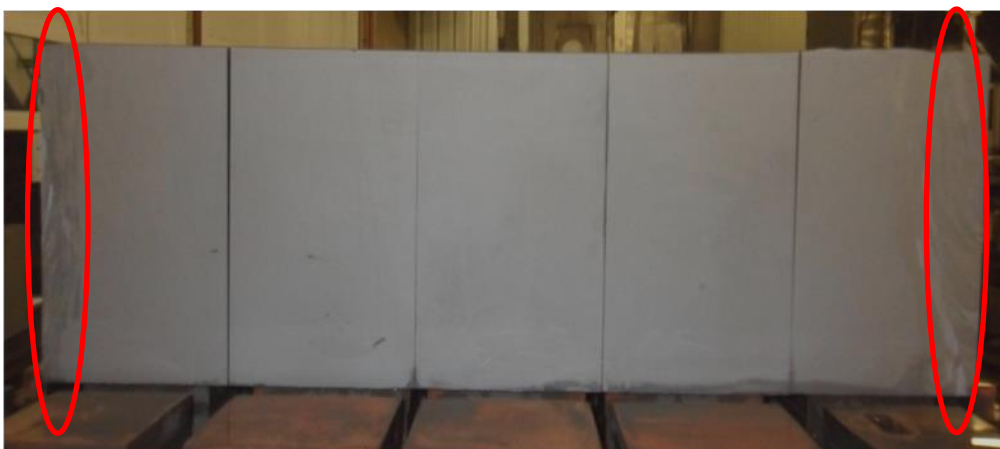
Figure 2-18: Bricks from different parts of an ingot showing a transversal cut. Red lines showing the multi crystalline due to the contact to the crucible walls. Reproduced from DCWafers.
