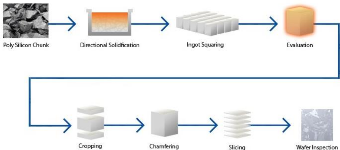
Figure 2-23: Schematic wafering process of casting ingots. Reproduced from Danen technologies.
