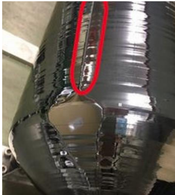
Figure 2-10: Ridges in the crystal surface of a dislocation-free ingot. Reproduced from [78].
