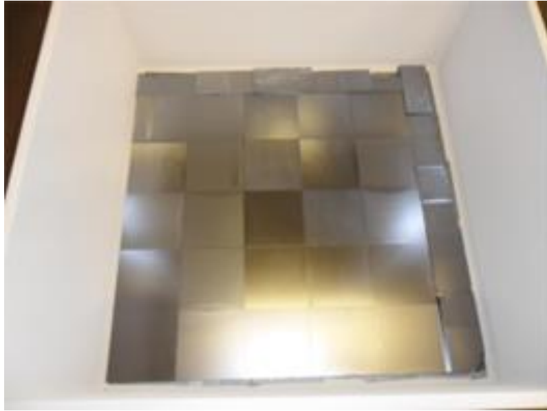
Figure 2-19: Several mono seeds charged in a crucible. Reproduced from DCWafers.
