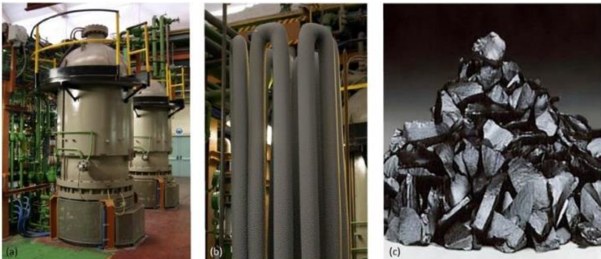
Figure 2-6: (a) Picture of a Siemens Reactor. (b) As grown polysilicon rods. (c) Final polysilicon chunks. Reproduced from [75].
