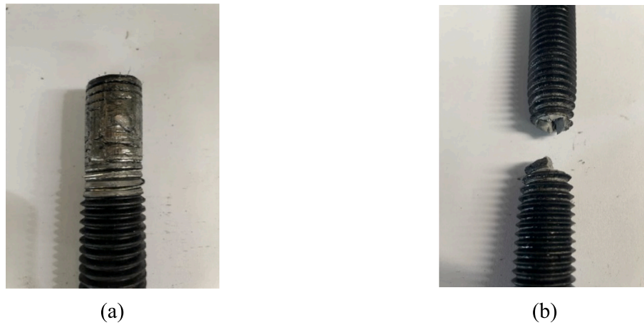
Fig. 13. Failure modes: (a) Thread stripping; (b) Bolt fracture.
