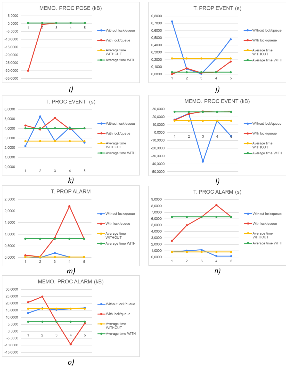
Figure 15. Propagation time, process time and memory used during process for the different messages: a), b) and c) Mission, d), e) and f) Mission report, g), h) and i) Pose, j), k) and l) Event and m), n) and o) Alarm.
