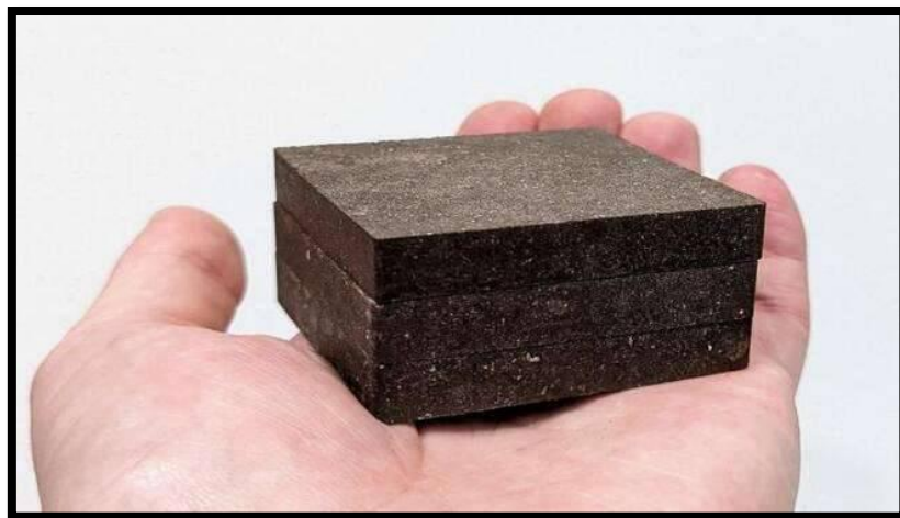
Figure 3.8: A Block Of Cusatis' Martian Concrete. (C&EN, 2023)
