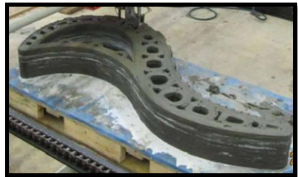
Figure 2. Construction with 3D printers with concrete (Source: Austin, Lim & Le, 2012)
