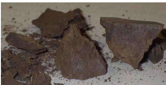
Figure 8. a sample of Martian concrete (Bob Yirka, 2016)
