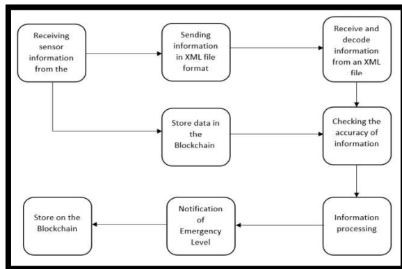
Figure 9: Flowchart of sending data to the central system
