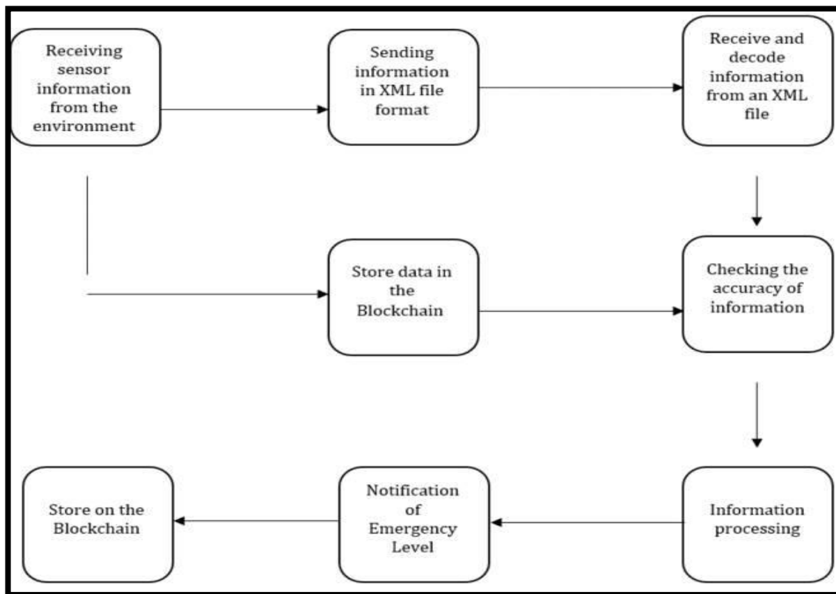
Figure 7.6: Flowchart Of Sending Data To The Central System (Author)
