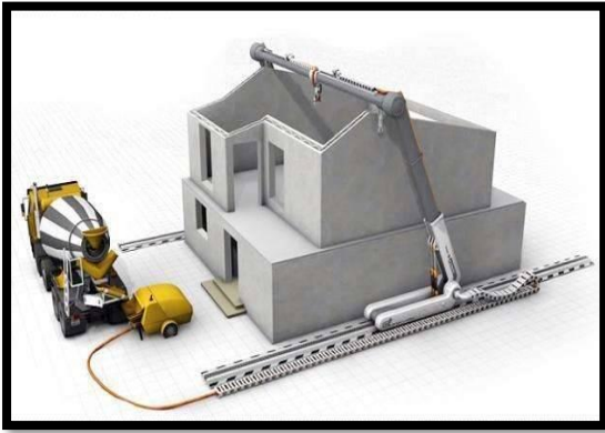
Figure 5. Construction of the Building by contour crafting (Source: Enzo Vergara, 2014)
