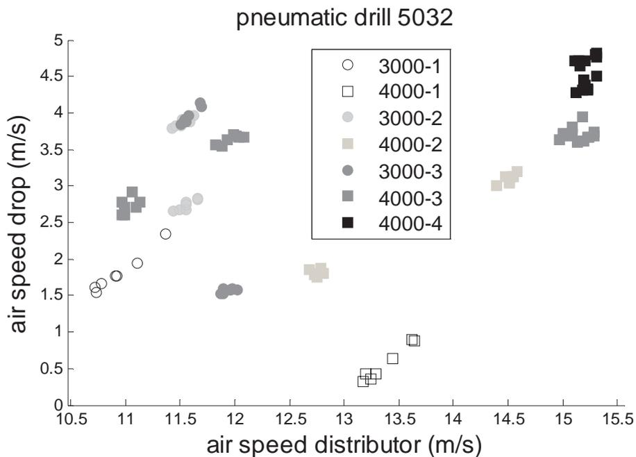
Figure 10. Scatter plot of air speed at the distributor compared to air speed drop in the seed pipe for seeders 5032.
