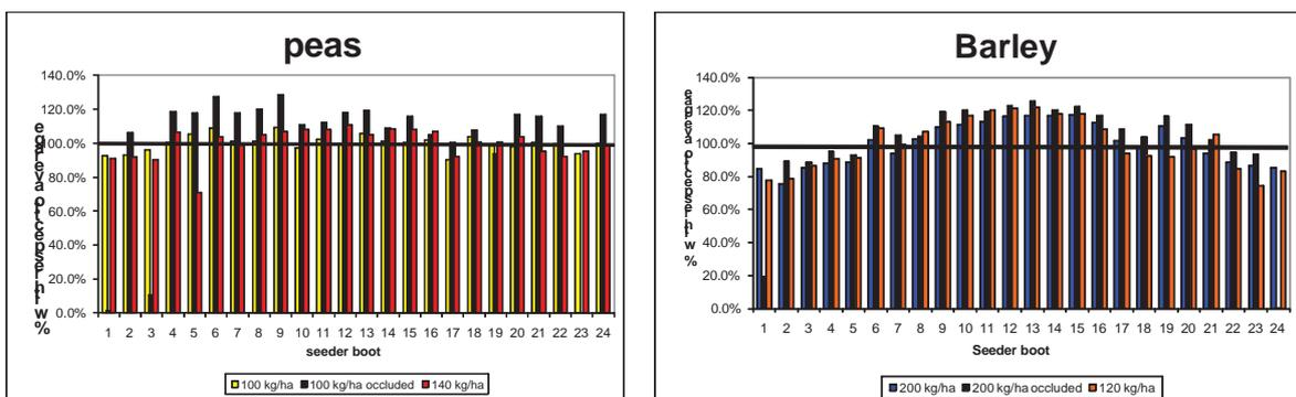
Figure 3. Comparison of transversal distribution with the same machine Pottinger Terrasem 3000 for peas (left) and barley (right) as referred by Gil-Quirós et al. (2007)
