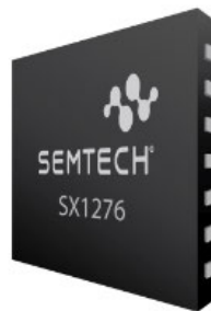
Figura 20: Chip SX127x de Semtech [29].
