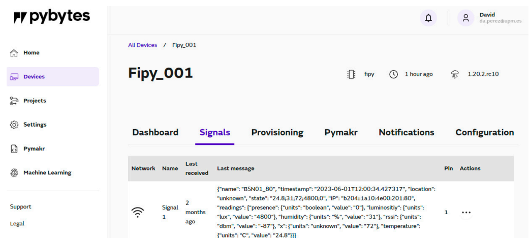
Figure 5. PyBytes’ back-end displaying the so-called Signals Table. The reader may see an example of one such message received from the Relay. In its structure, crucial pieces of information like the 6LoWPAN device’s identification, sensing values states, and measurement timestamps can be observed.
