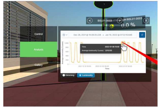
Fig. 6. Interaction with a line chart showing the average of the dimming values recorded by a streetlight during almost two weeks
