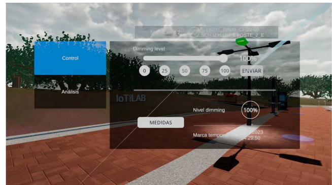
Fig. 1 – Screenshot illustrating the interface to control the dimming level of streetlights from the VR environment of the DT at University Campus de Montegancedo (Pozuelo de Alarcón, Madrid – Spain). All communication occurs in real-time to retrieve/update the status of the selected streetlamp as well as to show data and statistics to visualize (currently through the RESTful protocol only).
