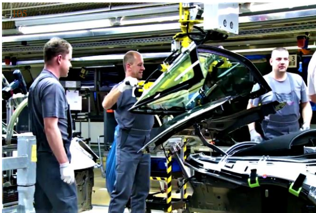
FIG.104-105: Factory Auto Glass Installation - 27 Oct 2017
