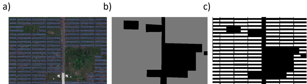
Figure 5.5: Solar panels dataset (Benhamadi, 2021; Jiang et al., 2021). a) Real aerial images b) Approximate ground truth provided in the dataset. c) Ground truth more precise built for this study.
